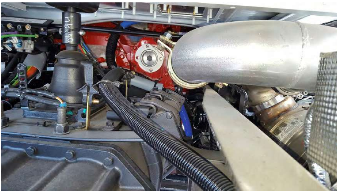
FIGURE 8-15. REPTO Flywheel Housing
