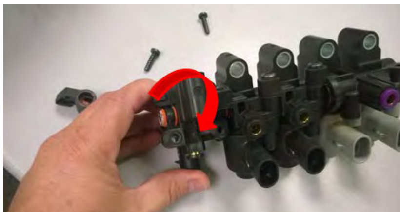
FIGURE 7-48. 23 EOa Solenoid Disassembly
