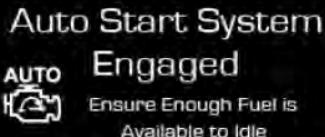
The fuel reminder message will be displayed after the Auto-Start Switch has been held to enable Auto-Start but before the system is fully enabled. Make sure there is sufficient fuel to run the engine.
