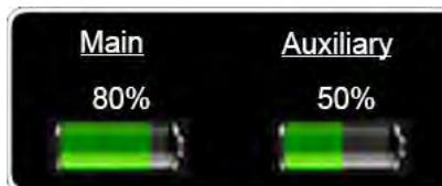
The Auto-Start system will display the State of Charge (SOC) of the vehicle's starting and auxiliary\* batteries while the batteries are charging. Auxiliary batteries are in the separate battery pack included with a factory installed electric air conditioning system. If SOC is not available, numerical percentage value will be replaced with "- -".
