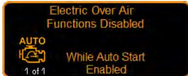
"XXXX" message will be displayed if any air-powered accessory switch is operated while the Auto-Start system is enabled.
