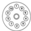
Nut Tightening Sequence for Stud Piloted Disc Wheels
