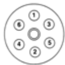
Nut Tightening Sequence for Stud Piloted Disc Wheels
