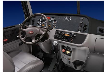
The rugged ProBilt interior features five grab handles, a powerful HVAC system and a charcoal colored dash made of durable materials that is easy to clean and shows less scratches and scuffs.
