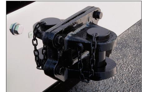
Bumpers on the Model 367 accommodate either a center tow hook configuration or a dual removable pin configuration that meet TMC towing guidelines of 80,000 pounds.
