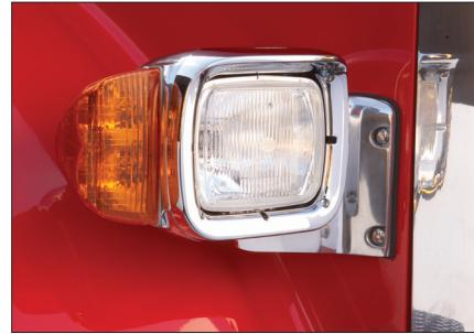
Pod-mounted headlamps are durable, corrosion-resistant and cost-efficient to replace. They feature halogen bulbs for 50% greater low beam performance and nearly 600% longer bulb life.
