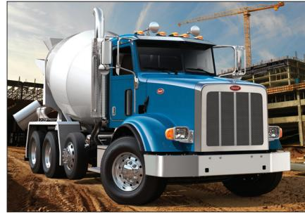
An advanced composite hood provides exceptional durability with a stainless steel grille to protect the cooling system. The hood design improves forward visibility.
