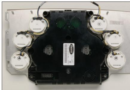
A multiplex electrical system offers diagnostic simplicity and reliability. The Electronic Service Analyst monitors the system, isolates sensors and gauges, and maintains an event log.
